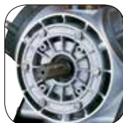
C/C Version 1 3/8" 6 Splined Thru Shaft
