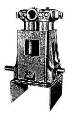
Royalette 2020 pumps are vertical, reciprocating, positive displacement, four piston pumps that deliver 20 gpm at up to 500 psi. The higher pressure in a 20 gpm pump gives finer spray droplet breakup for an enveloping type of spray coverage.
