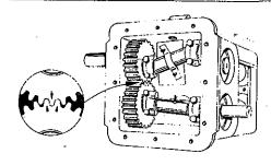
IMPORTANT-TIMING THE PUMP Arrows on gears must be located EXACTLY as shown above to properly time the pump.
