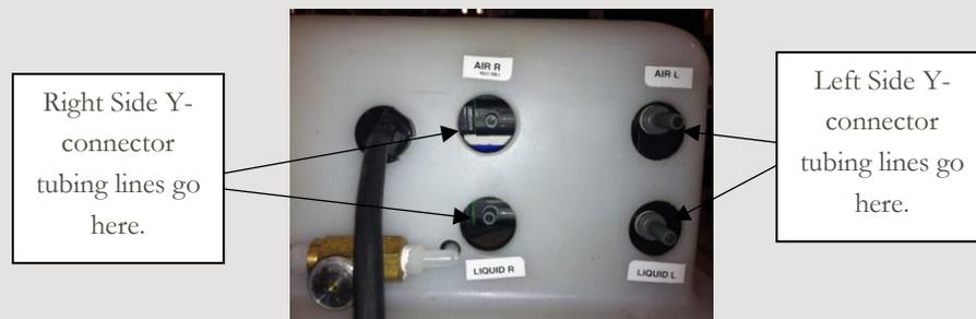
Finally, secure the tubing lines along the boom and sprayer frame with the nylon ties provided (NY108H). Be careful to not kink or pinch the lines with the ties provided. You should be ready to go! Make sure that your push to connect power chord is connected, and then follow our operating instructions to start making foam.
